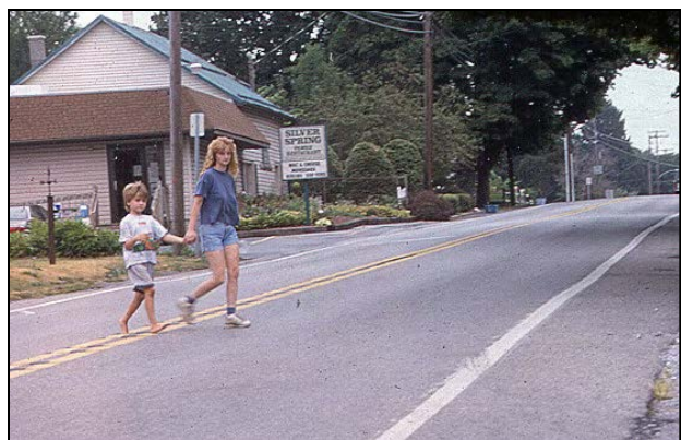
AVOID: Lack of crosswalk, speed limits, and warning signage all create a hazardous pedestrian situation (Silver Spring Village, West Hempfield Township, PA).
